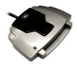
The ACR38 USB SAM from ACS is a high speed USB 2.0 smartcard reader containing a built in SAM (Security Access Module) slot. This reader is fully PC/SC and EMV Level 1 compliant and supports all ISO 7816 microprocessor-based smartcards as well as numerous popular memory cards.
